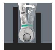
The Joker 6003 ring spanner with its special open end geometry open end offset by 7.5° and the double hexagon profile - doubles the placement possibilities when repeatedly turning the wrench 180° around the longitudinal axis. Bolts and screw heads can be "accessed" every 15°. The Joker 6003 will automatically find the respective placement point after every turn.
