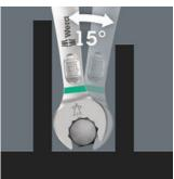
The Joker 6003 ring spanner with its special open end geometry - open end offset by  $7.5^{\circ}$  and the double hexagon profile - doubles the placement possibilities when repeatedly turning the wrench 180° around the longitudinal axis. Bolts and screw heads can be "accessed" every 15°. The Joker 6003 will automatically find the respective placement point after every turn.
